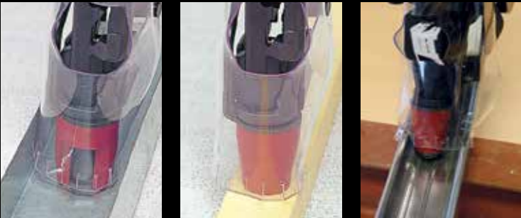
Metal track to concrete Wood track to concrete Metal track to steel
